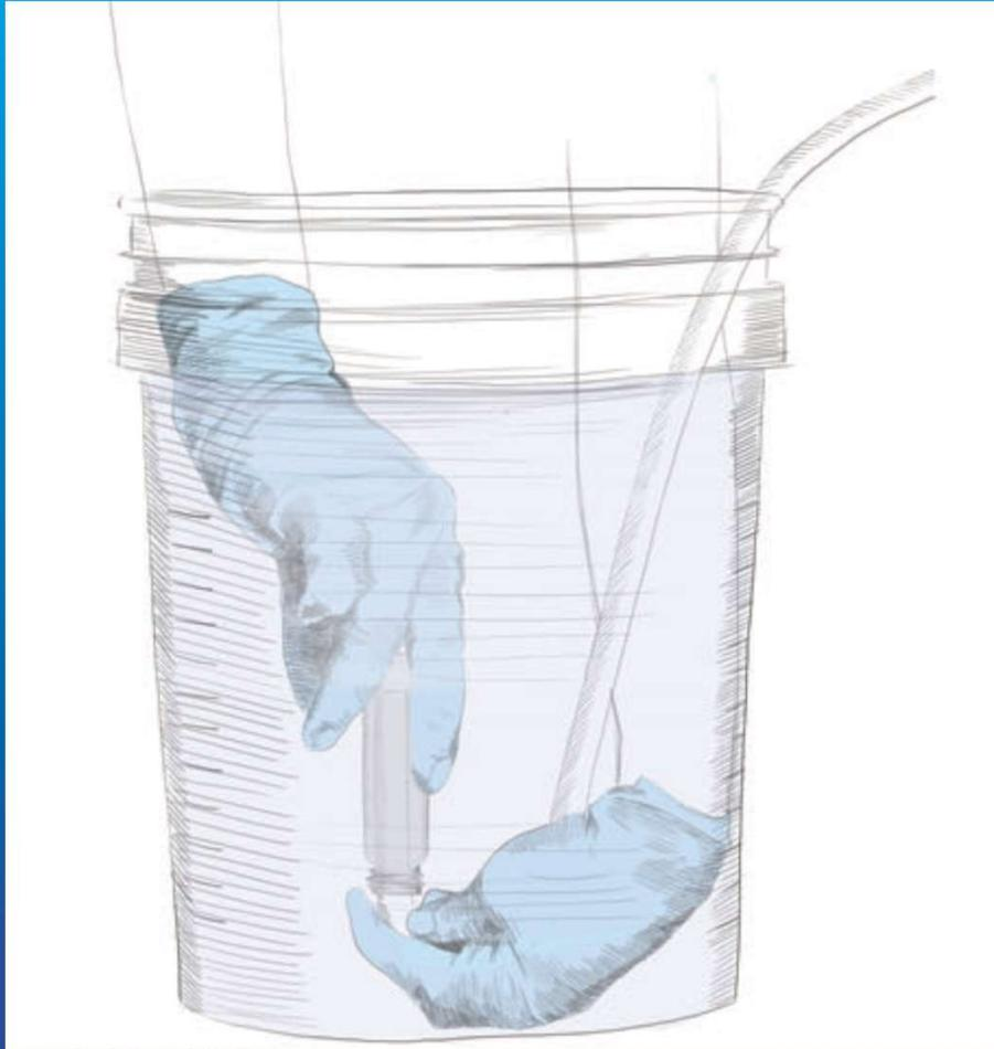
Inverted Fill – A VOA vial is inverted in a bucket of purge water and filled by displacement.
